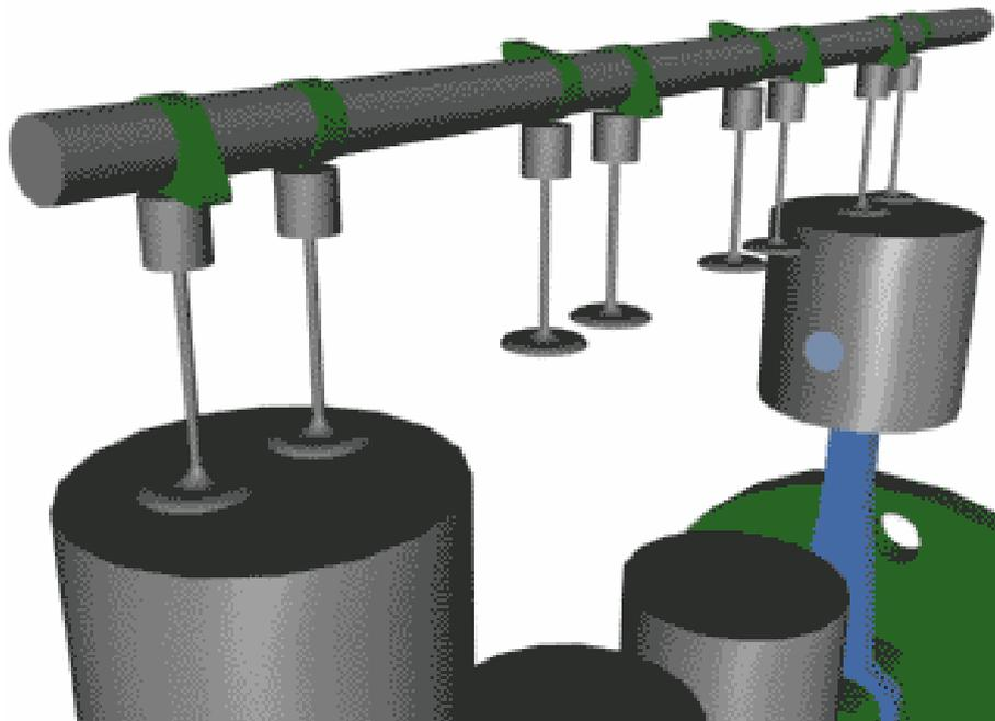
**Figure 6** The camshaft
