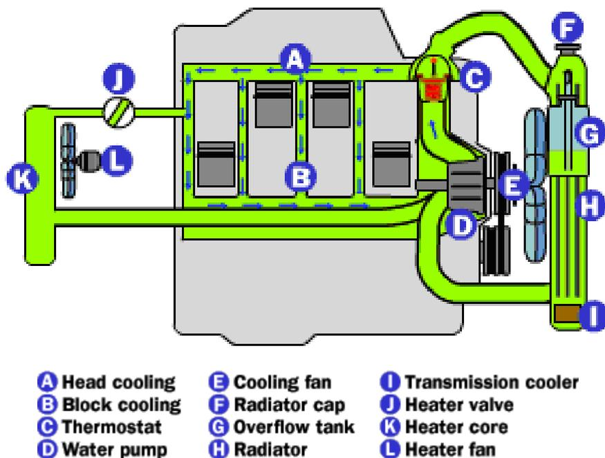
On cars with automatic transmissions, there is normally also a separate circuit for cooling the transmission fluid built into the radiator. The oil from the transmission is pumped by the transmission through a second heat exchanger inside the radiator.
