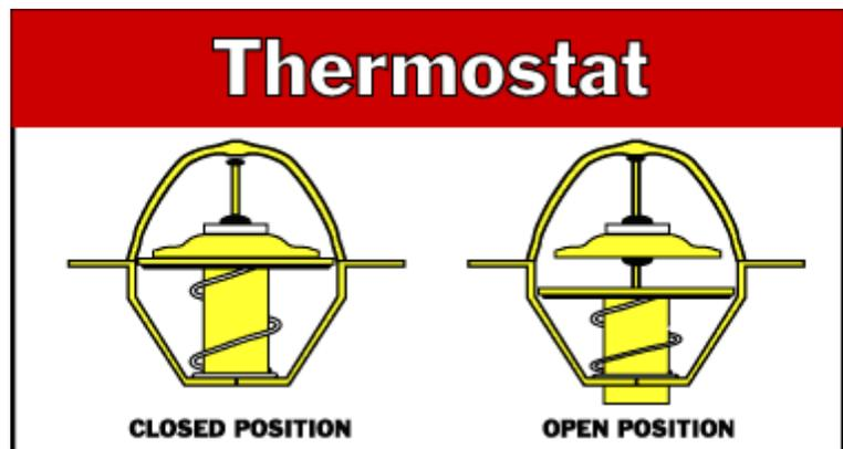
**The open and closed positions of a thermostat**
